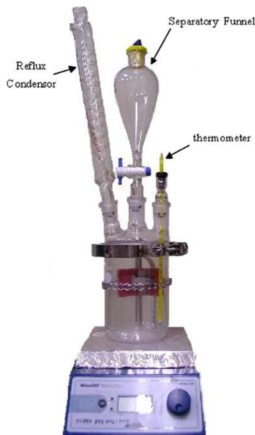
Fig. 1 Reflux system for preserving the concentration
